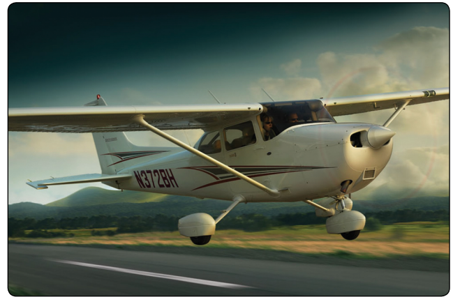
Figure 7-37. The landing gear supports the airplane during the takeoff run, landing, taxiing, and when parked.
