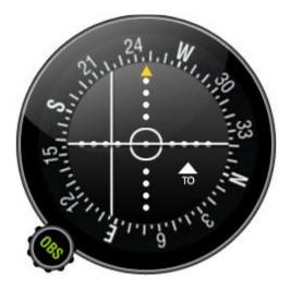
The VOR system is limited to about 1° of accuracy. One degree at 200 NM represents a width of: **A)** 3.5 NM.
