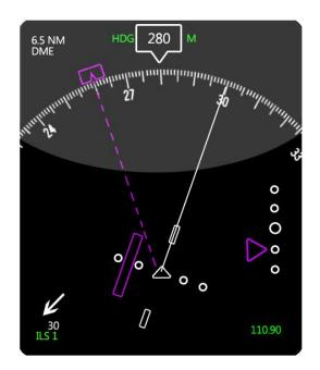
On a 2 dot EFIS HSI in the approach (APR) mode expanded scale what does one dot indicate? A)  $0.5^{\circ}$
